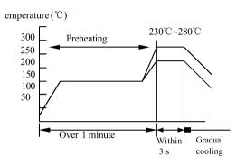
Recommended temperature for lead-free soldering
